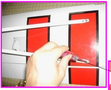
Install the wing supports with screws.
