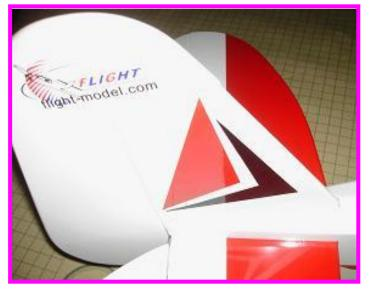
Insert the vertical fin and glue the rudder to the vertical fin .
