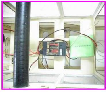
Assemble the receiver and receiver battery as shown.
