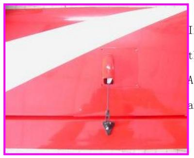
Install the servo cover to the bottom of the wings, and Assemble aileron, servo arm and pushrod.
