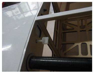
Insert the main wings with joiner, then screw them by nylon screws.
