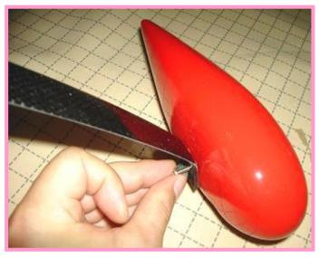
Permanently tighten the axle to the gear strut by wrenches.
