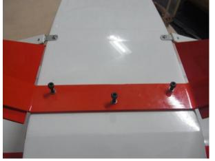
Install the undercarriage to the bottom of the fuselage.
