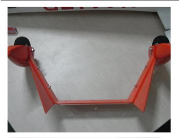
Install two wheels to the undercarriage as shown.
