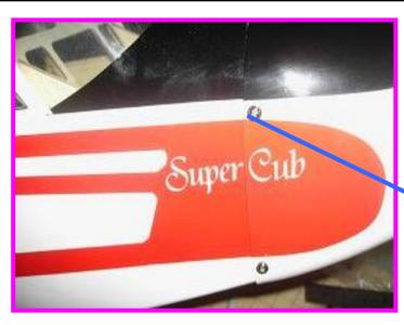
Install the cowling with screws which factory provided.
